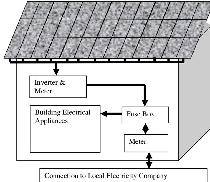
Figure 6.2 – schematic of grid connected renewables
