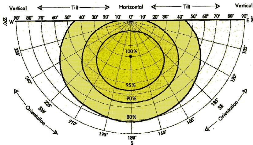
Figure 6.4 – orientation losses for a PV system
