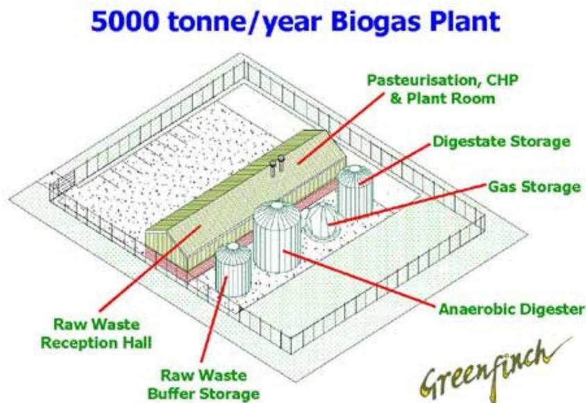
Figure 6.11 – Biogas food processing plant, courtesy of Greenfinch
