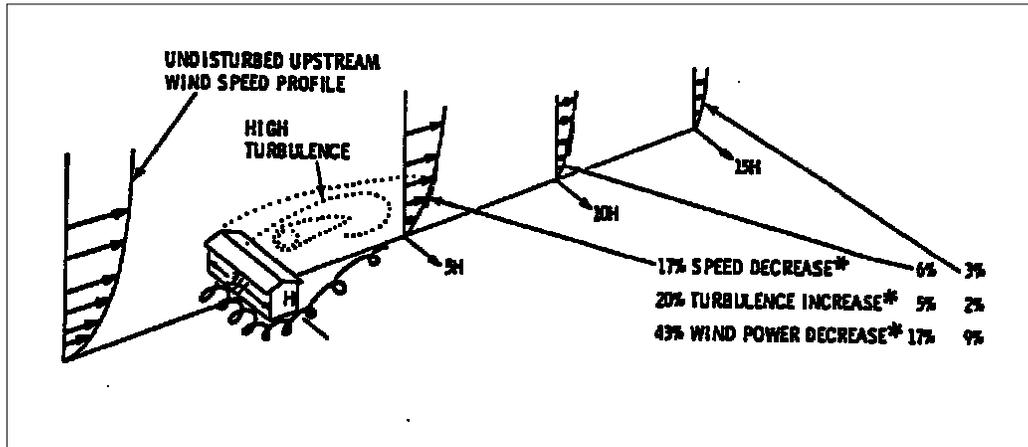
Figure 6.8 - Effect of turbulence on wind power, from Wegley
