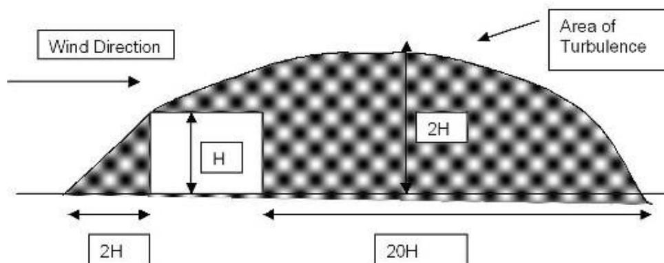
Figure 6.7 – Area of turbulence caused by object
