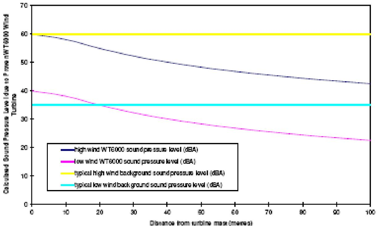
As can be seen the turbine noise quickly becomes less than the background noise. As other habitation is more than 250m away we can expect noise levels from the turbine to be 34dBA in high wind speeds. To put this into some perspective the table overleaf gives typical noise levels for different situations.
